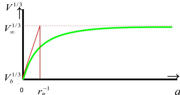
$$V^{1/3}(a) = V_\infty^{1/3} - (V_\infty^{1/3} - V_b^{1/3}) \exp(-r_B a)$$
